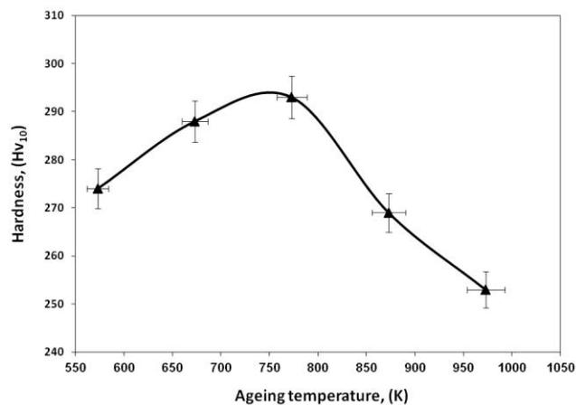
**Figure 6: Hardness Measurements versus Ageing Temperature**
