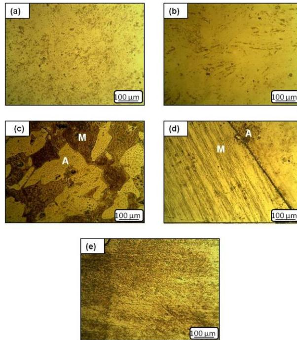
**Figure 2: Microstructure of Aged Ni<sub>51</sub>Fe<sub>18</sub>Ga<sub>27</sub>Ti<sub>4</sub> Alloy for 3 h at (a) 573 K (b) 673 K (c) 773 K (d) 873 K and (e) 973 K**
