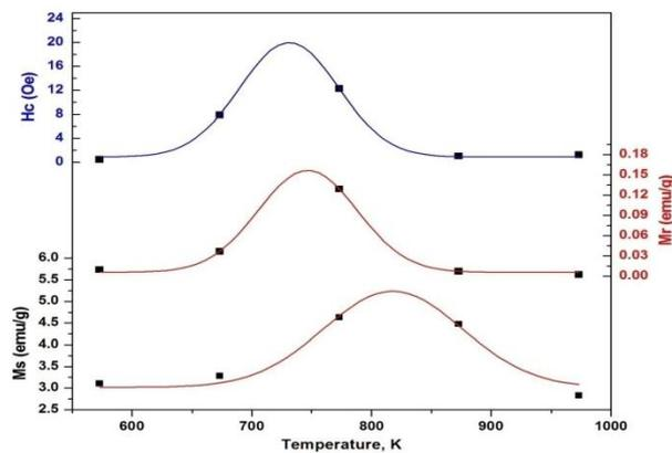
**Figure 5: Effect of Ageing Temperature on the Saturation Magnetization ( $M_s$ ), Remnant Magnetization ( $M_r$ ) and Coercivity ( $H_c$ ) of Ni<sub>51</sub>Fe<sub>18</sub>Ga<sub>27</sub>Ti<sub>4</sub> Alloys**
