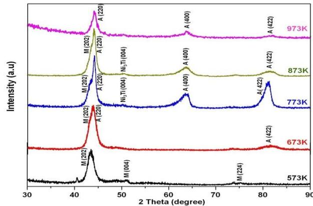
**Figure 1: XRD Patterns at Room Temperature of Ni<sub>51</sub>Fe<sub>18</sub>Ga<sub>27</sub>Ti<sub>4</sub> Alloy Aged at 573-973 K for 3 h**
