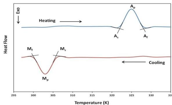
**Figure 3: Martensitic and Austenitic Transformations at 773K for 3 h**
