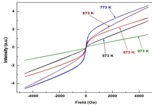
**Figure 4: Magnetization Saturation of Aged Ni<sub>51</sub>Fe<sub>18</sub>Ga<sub>27</sub>Ti<sub>4</sub> Alloys**
